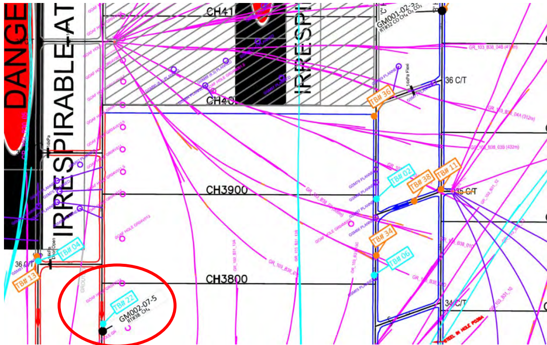
Figure 85: Extract from ventilation plan from June 2020 showing the 400 metre CH 4 sensor (GM002-07-5) and TB #22.
