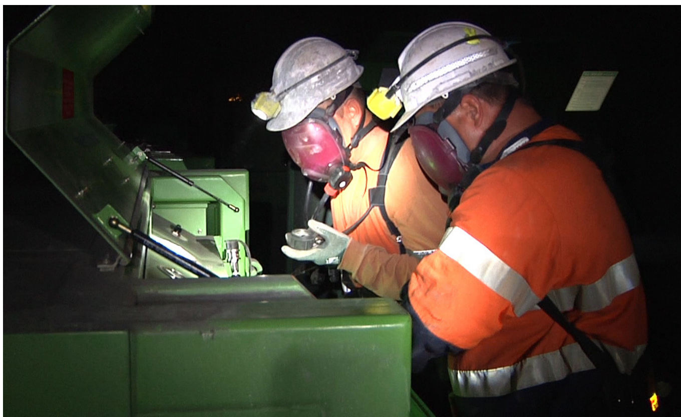
Coal mine workers top up their CABA and check the fill gauge during the 2014 level 1 exercise Photo: DNRM
