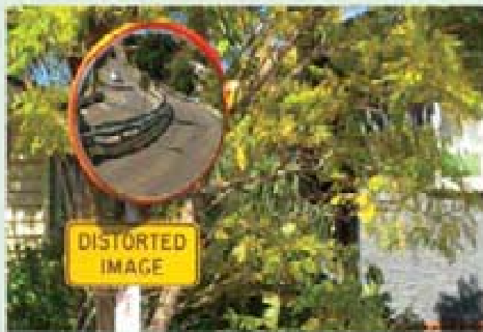
→ Convex mirror installed to improve road safety
