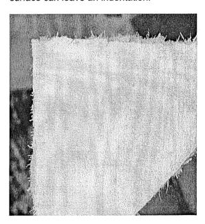
Photograph 2: Low density asbestos fibre board
